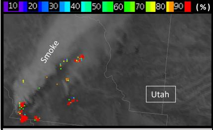
Suomi NPP VIIRS-AF overlaid onto GOES-16 0.64  $\mu m$  visible imagery, observing wildfires and smoke in Utah at 2020 UTC on 19 September 2018. The colors represent detection confidence (%), while the size of the dots increases with FRP.
