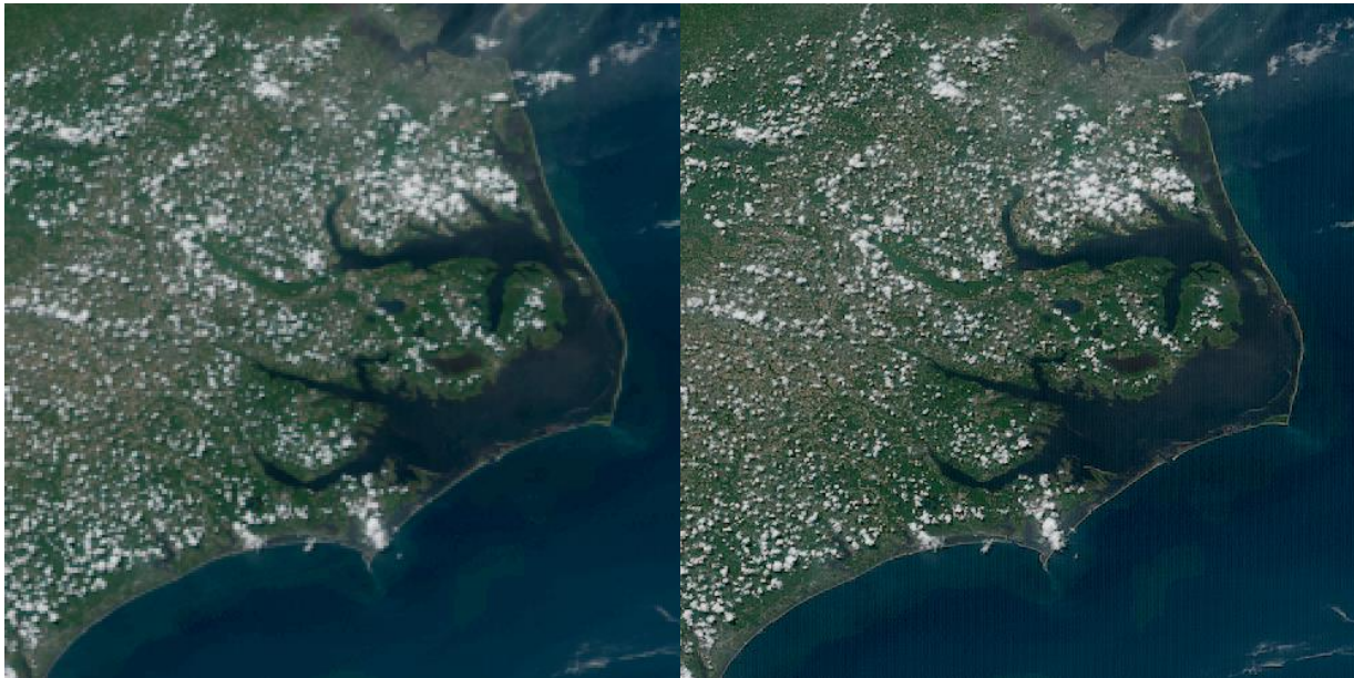
Figure. GeoColor images produced at 1 km resolution (left) and 500 m/HKM resolution (right) over eastern North Carolina (18:25 UTC, 1 June 2022).
