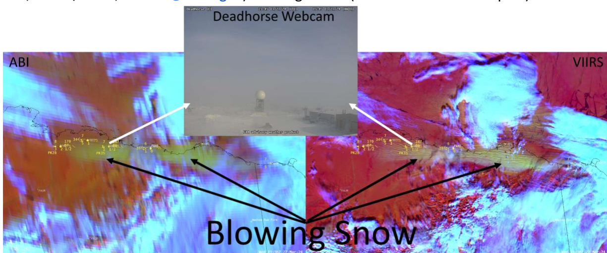
Figure: 27 March 2024 GOES-18 ABI (left) and VIIRS (right) Blowing Snow RGB over far northern Alaska, from AWIPS. Deadhorse, AK webcam view from within the blowing snow, showing significantly reduced visibility.
