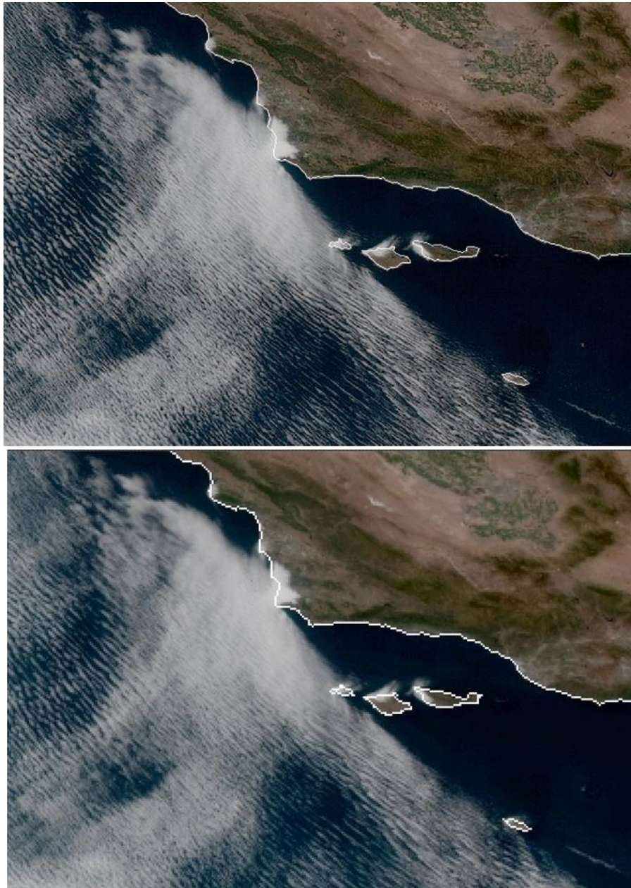
Figure M1-1: Comparison between half-kilometer (HKM, on top) and 1-km (bottom) resolution versions of GeoColor from GOES-17 (23:30 UTC, 30 June 2019).
