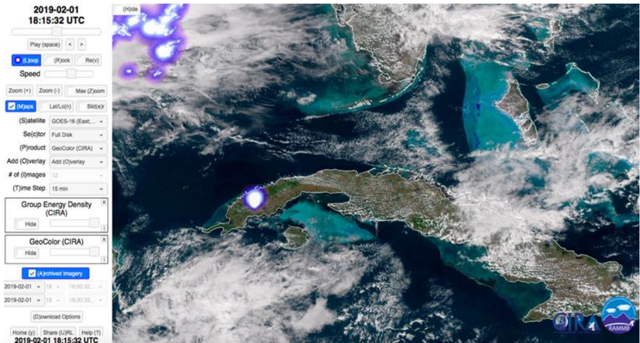
Figure M3-1: GLM-detected asteroid flash over Cuba, as shown by RAMMB/CIRA SLIDER on 1 February 2019 at 18:15:32 UTC. The image is GOES-16 ABI GeoColor with the GLM Group Energy Density overlay.
